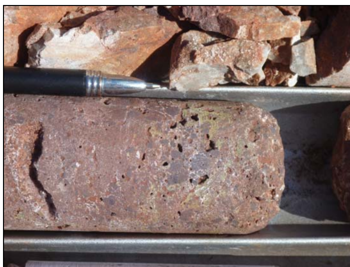
Reworked hematitic gossan in drill core, containing the copper-lead-zinc vanadate mineral mottramite (yellow-green).
