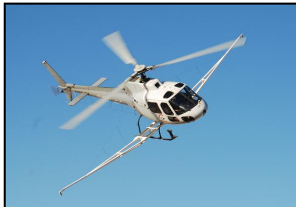
Figure 2 – The contract helicopter with dual sensor boom attachment for recording magnetic and radiometric data.
