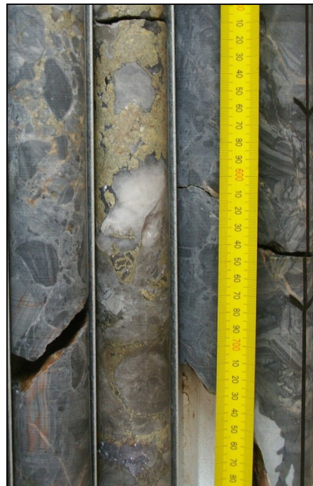
An example of strong zinc and lead sulphide mineralisation within drillhole BDDD0023 (~118m)
